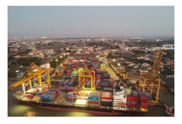
Higher Container loading/discharging rates through better handling equipment 3x35-tons quay cranes and specially well trained equipment operators with productivity of 25 moves/hour/crane ensures punctual vessel schedule.
