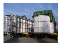
Steel Tonnage 267 tonnes Shipping Weight 1,630 tonnes Coil Materials A106, SS310, SS04, P22 HP40 modified + Nb Owner Thai Olefins Employer Chiyoda Corp Location Maptaphut, Thailand Completion Date December 2003
