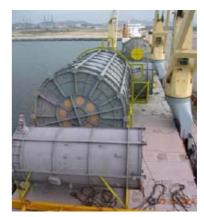
Steel Tonnage 214 tonnes Shipping Weight 929 tonnes Coil Materials A106, P9, P22, P11, P5 Owner Pertamina / Toyo EC / PT Rekayasa Industri Employer Furnace Engineering Location Balongan, Java, Indonesia Completion Date April 2004
